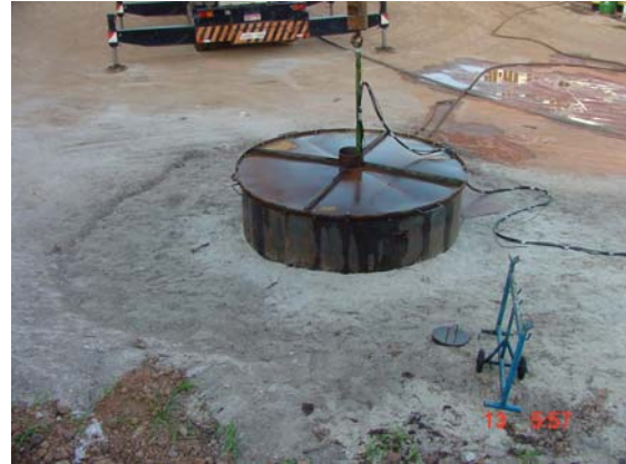
Figure 4 - Metallic pit used to shoot the airguns. Note the stability of the set, either after more than five hundreds shots.
