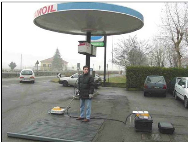
Fig.5. A 3D acquisition using the PSG with a 500MHz antenna.
