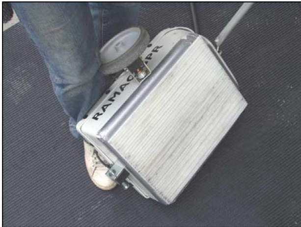
Fig.4. Pad System for Georadar (PSG).
