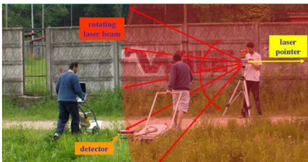
Fig.9. Application of the laser-beam system for archeological investigations with a 250MHz antenna.
