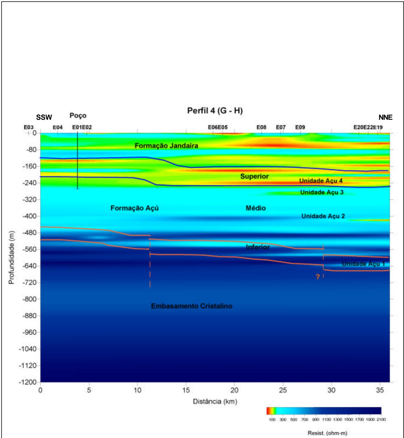
Figure 4 – 2D Hydrogeological Model based on the 2D Pseudo Goelectrical Section of the SSW-NNE Perfil in the Plataforma de Aracati region of the Potiguar Basin.
