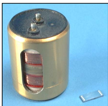
Figure 2: Conventional Geophone and a Digital MEMS Sensor
