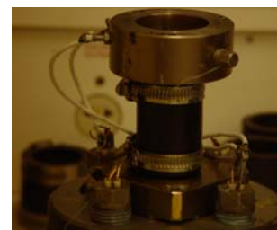
Fig. 3b – The sample inside the rubber jacket, ready to go to the pressure vessel.
