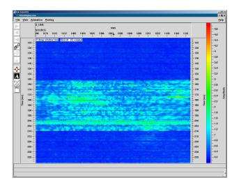
The RMS display shown above illustrates the extreme sensitivity of the crossline geophone to above-mudline events. The 6km cable is represented by the vertical axis with time along the horizontal axis. The upper 2 kms of cable were trenched to 2 metres, the middle 2 kms were left on the surface of the seabed whilst the lower 2kms were trenched to 1 metre.
