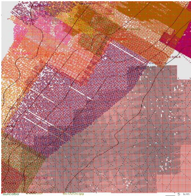
Figure 9 – Map showing the new velocity locations (red dots) after collection, gathering, stacking and smoothing. In this case it was used a 500 x 500 m cell size. The original velocity locations (see figure 8) are underneath.
