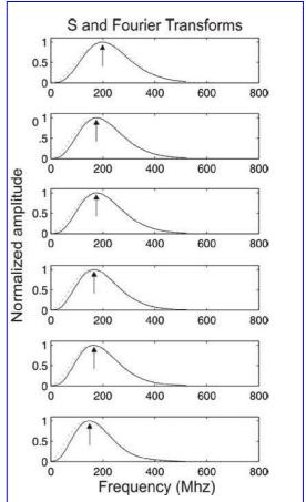
Figure 3: comparaion of S-transform (continuos line) with Fourier (dotted line) amplitutide spectra for the six arrivals of trace shown in Figure 2. The arrows identifies the centroid peaks.
