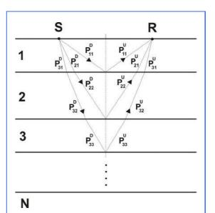
Figure 1: stratified earth composed of N layers showing ray paths from source S to receiver R.
