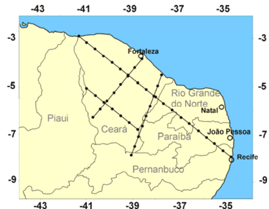
Figure 10. Interlinked refraction lines, a probable layout of refraction lines in the NW-SE transect in Borborema Province
