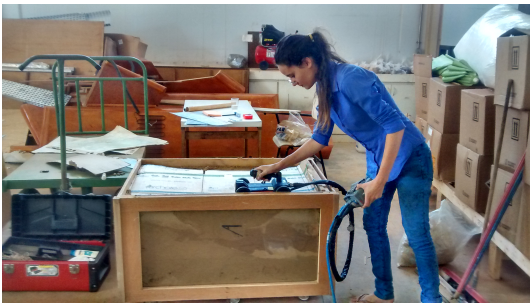
FIG. 1. GPR acquisition on a sand box.
