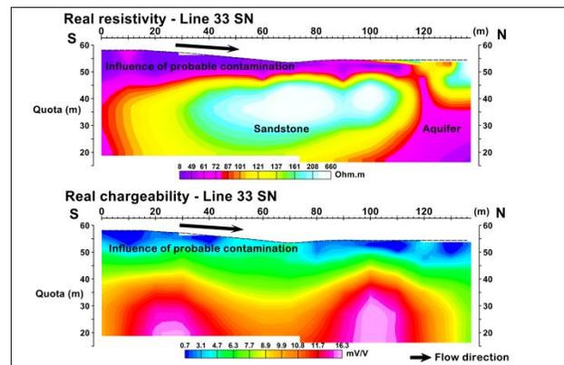
Figure 4 - Resistivity and chargeability 2D depth models of the Line 33 SN (see location in Fig. 2)
