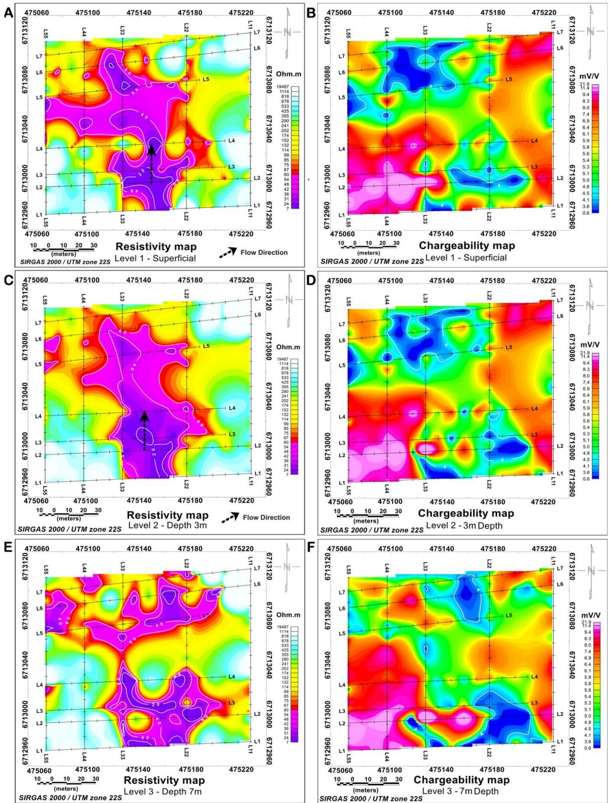
Figure 5 - Resistivity (A, C, E - superficial, depth 3 m and depth 7m, respectively) and chargeability maps (B, D, F - superficial, depth 3 m and depth 7m, respectively).
