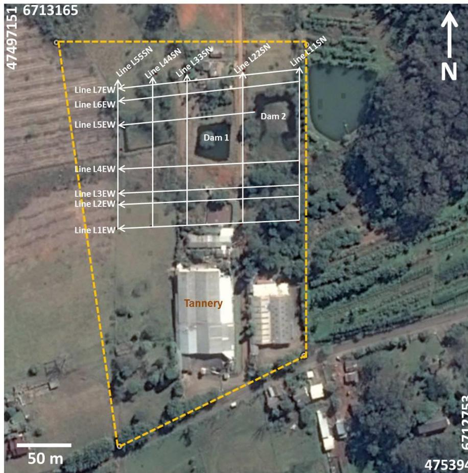
Figure 2 – Map of the study area, indicating the survey lines of geophysical methods (electrical resistivity and induced polarization). Google Earth (2015).
