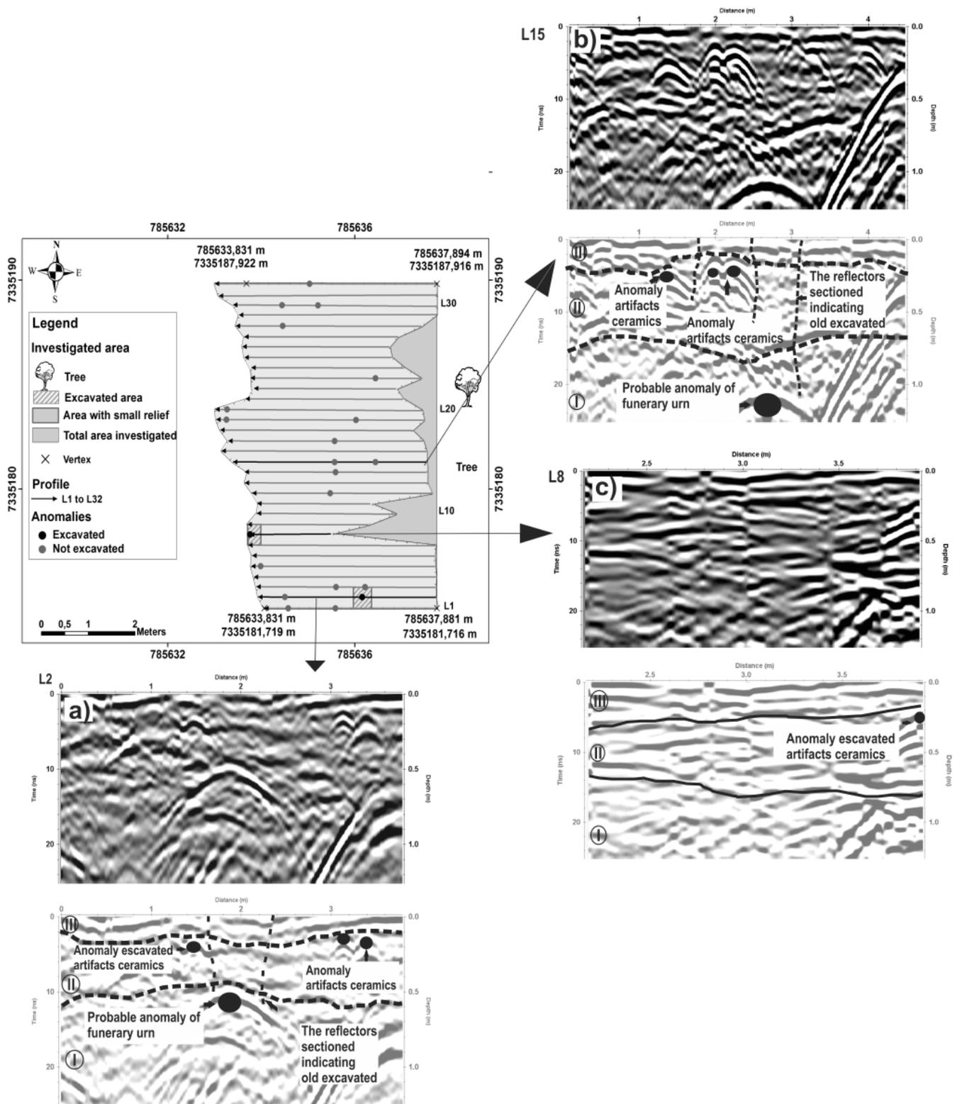
Figure 3 - Results of sections 2D characterizing the anomalies evidenced at the site.
