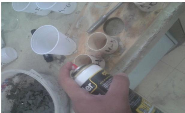
Figura 1: This picture, shows the vaseline spray being passed in the bottle to make it easy to remove the sample.
