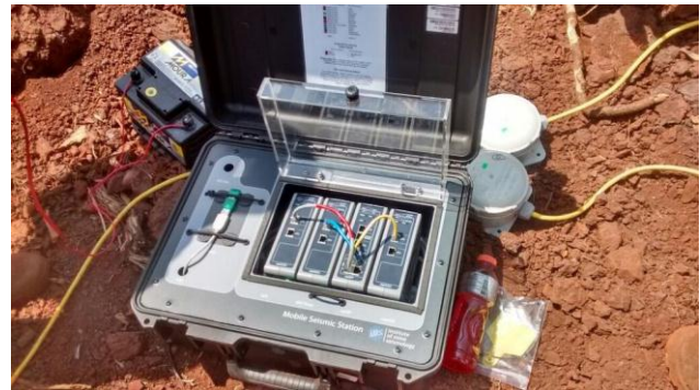
Figure 4 – Mobile seismic station used to record continuous vibrations measured by the geophones.
