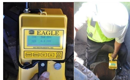
Figure (3) Measurements of methane concentrations in water wells.
