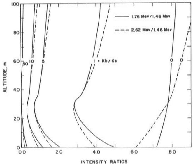
Figure 4 - Calculated intensity ratios versus altitude of detector for some typical ratios between potassium in total dry biomass (Kb) and mineral soil (Ks). For these curves we considered the same concentrations employed for Figure 3.
