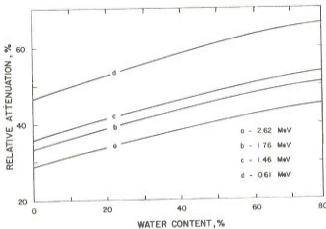
Figure 5 — Calculated relative attenuation of gamma photons versus water content of stand forest and roots. For calculating these curves the radioisotopic concentrations were taken as zero in the total biomass, and unit in the mineral soil.
