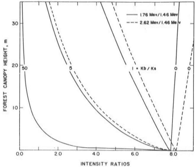
Figure 3 - Calculated intensity ratios versus height of forest canopy for some typical ratios between potassium concentration in total dry biomass (Kb) and in the mineral soil (Ks). For these curves Ks is constant and equal to 0.01%. Both eU and eTh are taken to be 1 PPM in the mineral soil and zero in the entire biomass.
