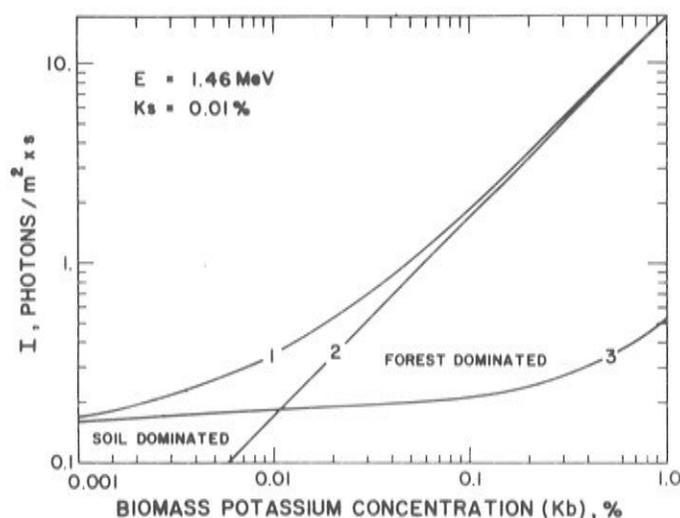
Figure 7 — Intensity of 1.46 MeV photons calculated for 100 meter flight altitude versus concentrations of potassium in total dry biomass. Curve 1 shows the total intensity, curve 2 represents the forest generated component and curve 3 shows the soil generated component (including roots and dead biomass).
