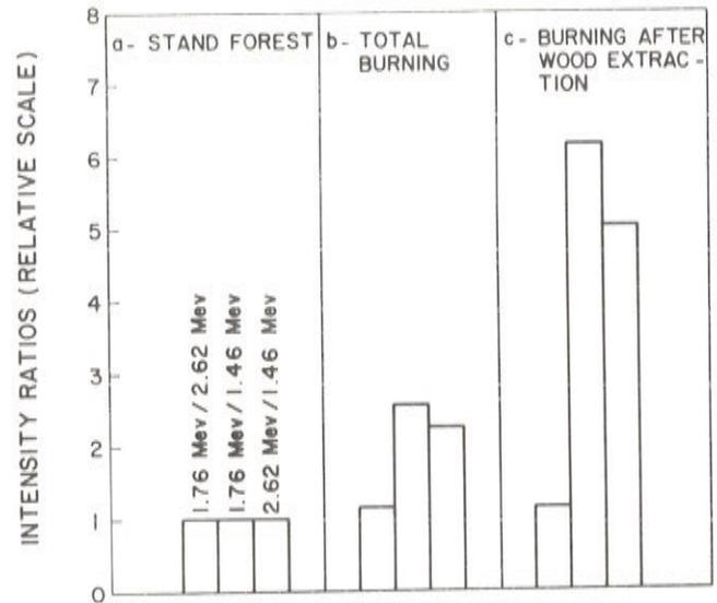
Figure 6 — Calculated effects of forest clearings on the airborne measured gamma-ray intensity ratios. For the calculation we have assumed eU and eTh concentrations of 1PPM in the mineral soil and zero in the biomass. Potassium was taken as 0.001% in the mineral soil and 0.1% in the biomass. The intensity ratios shown here are all normalized for the stand forest values.
