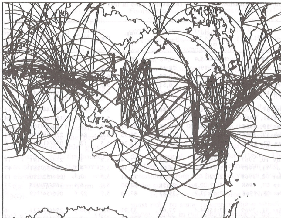
Figure 12. Geographical distribution of great circle paths corresponding to the references period 50 sec of our database of published phase velocity data. The latitude ranges from 75°N to 70°S in the map.
