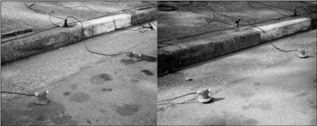
Figure 2 – Deployment of geophones with clay and metal base.
