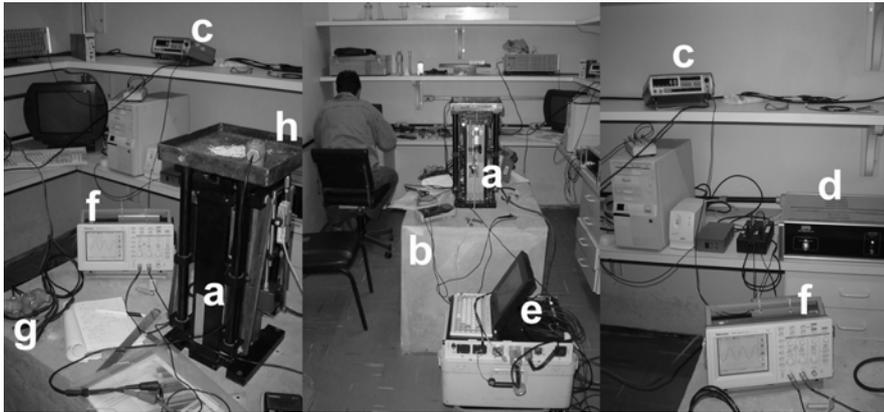
**Figure 5** – Design of shake table test: (a) APS Dynamics Inc. shake table (APS Electro-six model); (b) massive block of concrete; (c) Entelbra audio generator (ETB511 Model); (d) APS Dynamics Inc. Power Amplifier signal amplifier (124 model); (e) OYO-1 seismograph; (f) Tectronix oscilloscope (TDS220 Model); (g) four 100 Hz geophones; (h) geophone “tray”.
