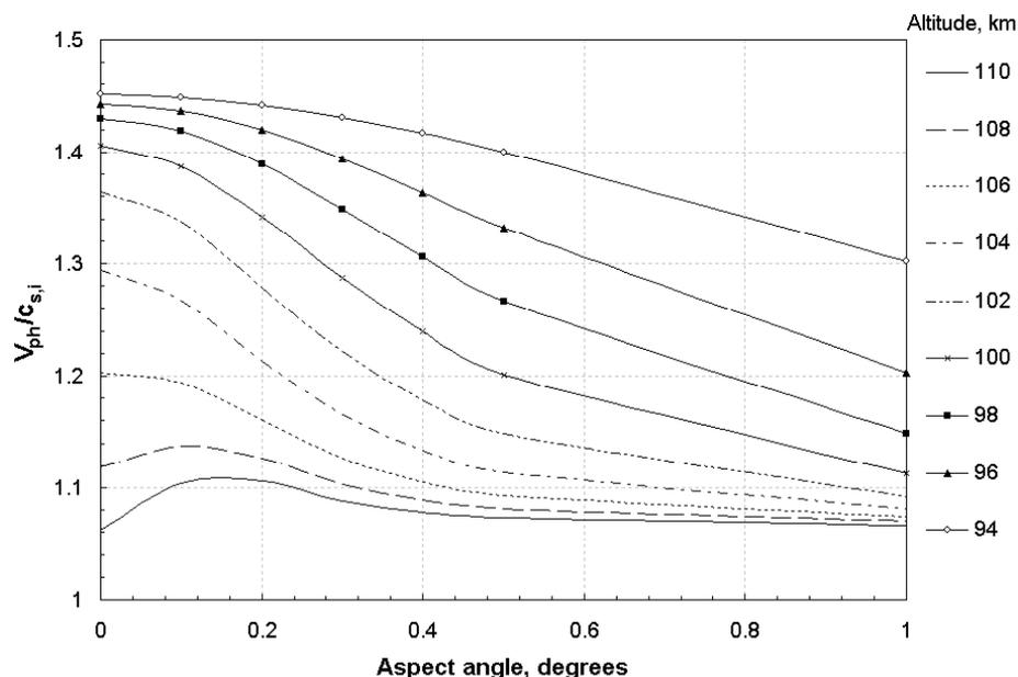
**Figure 3** – Variations in the ratio of the threshold phase velocity to the isothermal ion-acoustic speed as a function of aspect angle and altitude. An aspect angle of 0.25 deg or less means substantially greater threshold speeds between 100 and 106 km altitude. The aspect angle is not so influential lower down. From Kagan & St.-Maurice (2004).
