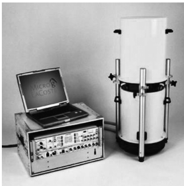
Figure 2 – Micro-g LaCoste absolute gravimeter A-10: repeatability and accuracy of 0.01 mGal on a quiet pier. High capacity battery for field operation not shown.
