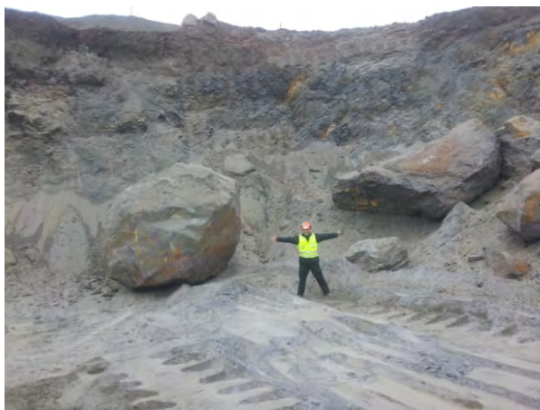
Figure 1 – Compact itabirite blocks immersed in friable material after a blast in a production bench at Abóboras mine.
