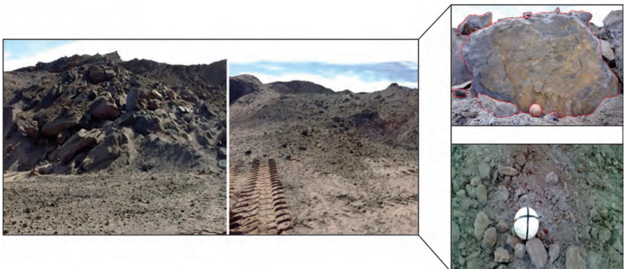
Figure 16 – Photographs illustrating the improvement in the fragmentation of the material produced by the fragmentation at the Abóboras mine.
