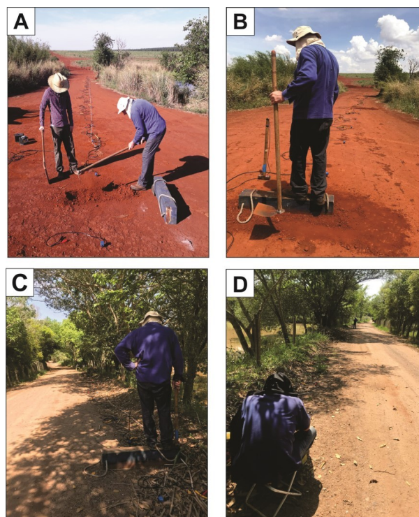
Figure 5 - A) Preparation of the S-wave source site for the seismic refraction essay; B) Arrangement and seismic data acquisition in Cordeirópolis – São Paulo; C) Seismic survey in the dam in Ipeúna – São Paulo; D) Seismic data acquisition in Ipeúna – São Paulo.
