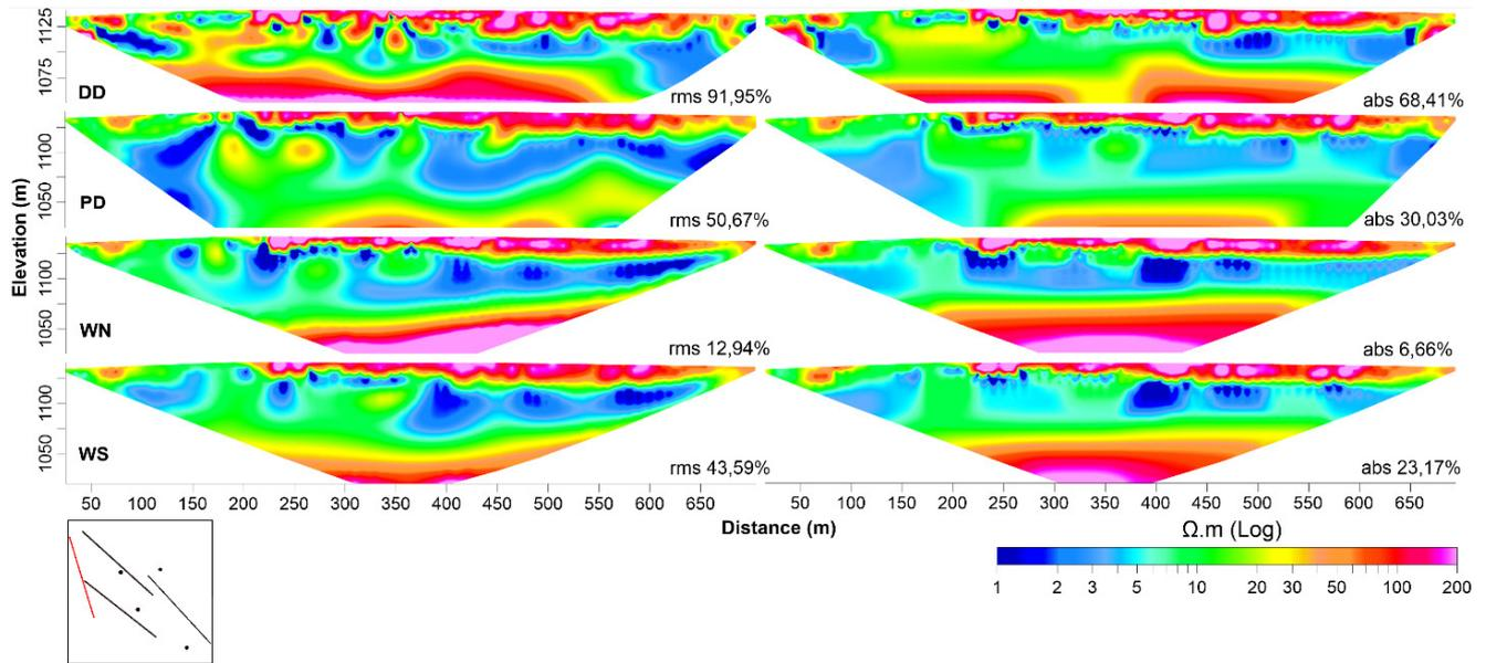
**Figure 4** - Comparison between resistivity sections for line L2 obtained with the four arrangements. On the left, the sections after inversion by the L2-norm method, with errors in RMS; and to the right, sections after inversion by the L1-norm method, with absolute errors.
