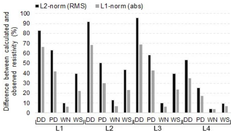
**Figure 7** - Misfit errors for models inverted by L1-norm and L2-norm methods for all ERT lines and all array configurations.
