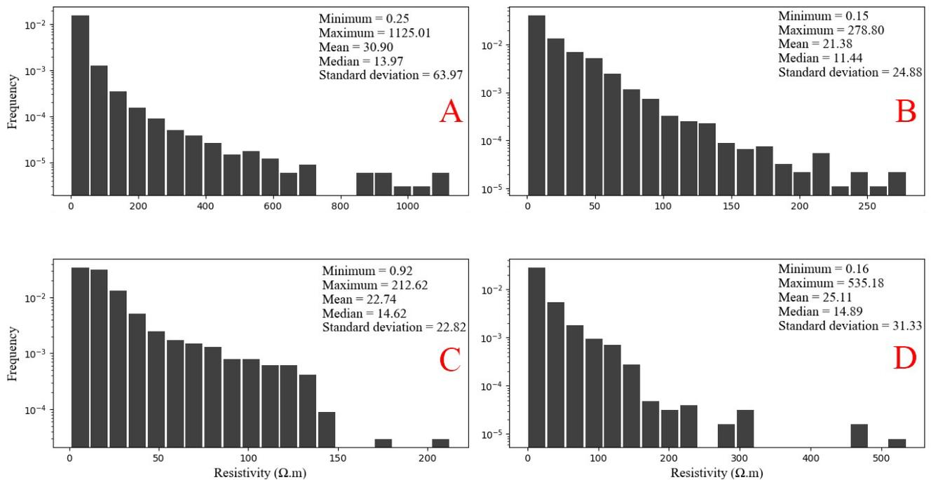
**Figure 2** - Histograms of the grouping of all distributions of filtered data. A) All dipole-dipole acquisitions; B) All pole-dipole acquisitions; C) All Wenner acquisitions; D) All Wenner-Schlumberger acquisitions.
