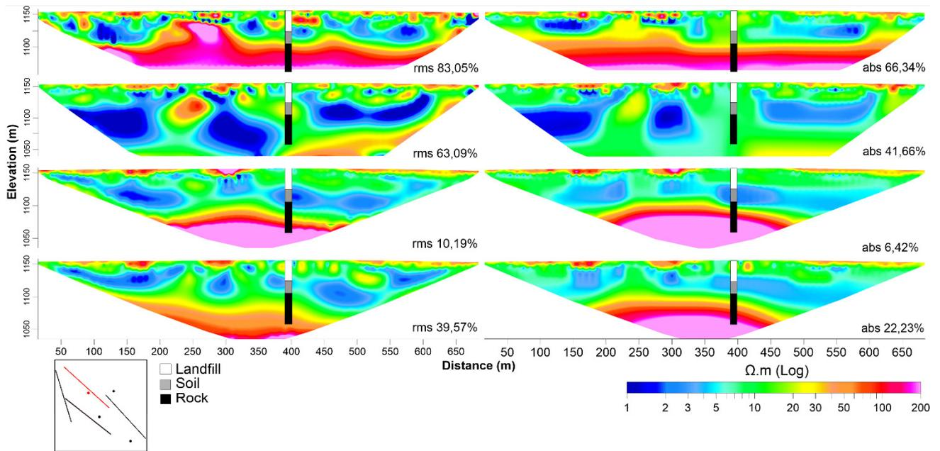
**Figure 3** - Comparison between resistivity sections for line L1 obtained with the four arrangements, with borehole B2. On the left, the sections after inversion by the L2-norm method, with errors in RMS; and to the right, sections after inversion by the L1-norm method, with absolute errors.
