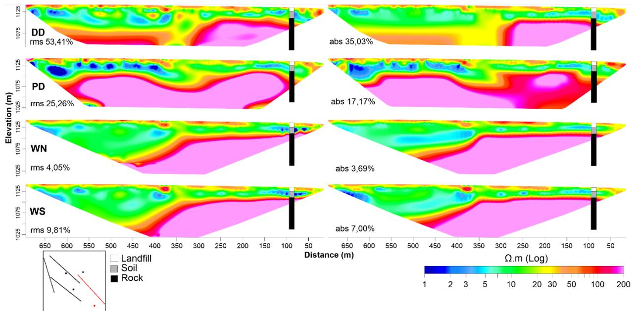
**Figure 6** - Comparison between resistivity sections for line L4 obtained with the four arrangements, with borehole B1. On the left, the sections after inversion by the L2-norm method, with errors in RMS; and to the right, sections after inversion by the L1-norm method, with absolute errors.
