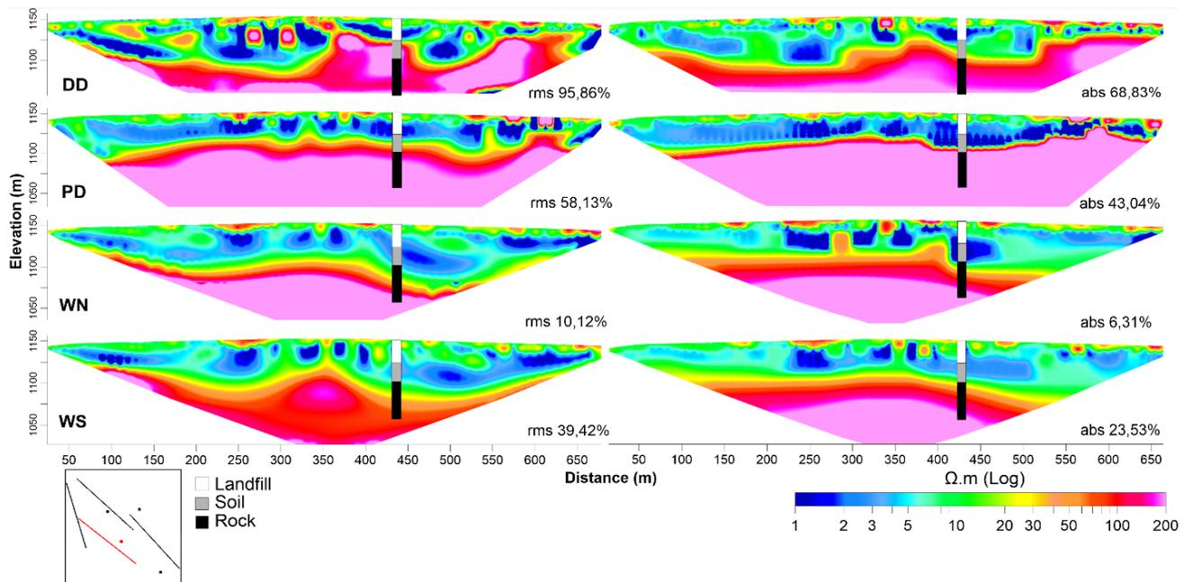
**Figure 5** - Comparison between resistivity sections for line L3 obtained with the four arrangements, with borehole B4. On the left, the sections after inversion by the L2-norm method, with errors in RMS; and to the right, sections after inversion by the L1-norm method, with absolute errors.
