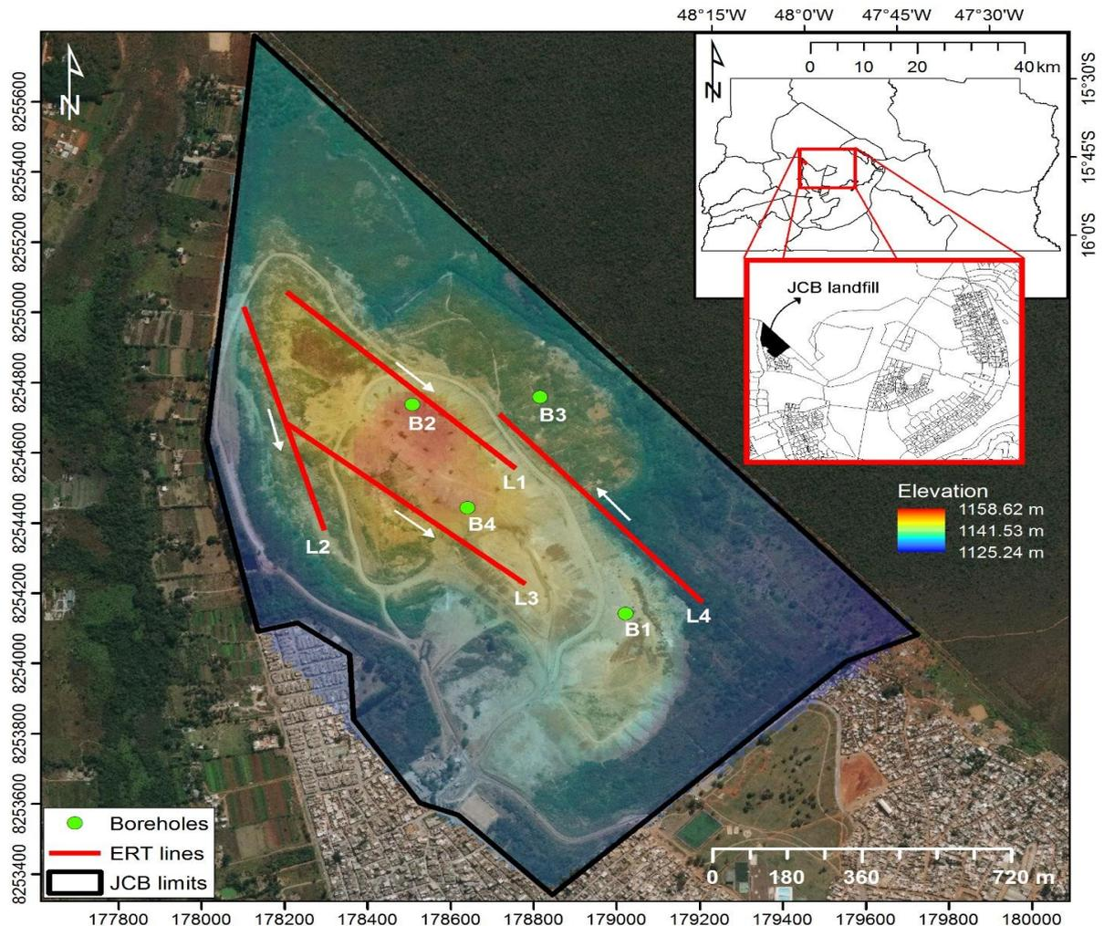
**Figure 1** - Location map of the Federal District of Brazil. ERT lines and boreholes at the JCB landfill, with area elevation and the study area limits. The white arrows indicate the direction of the data acquisition.
