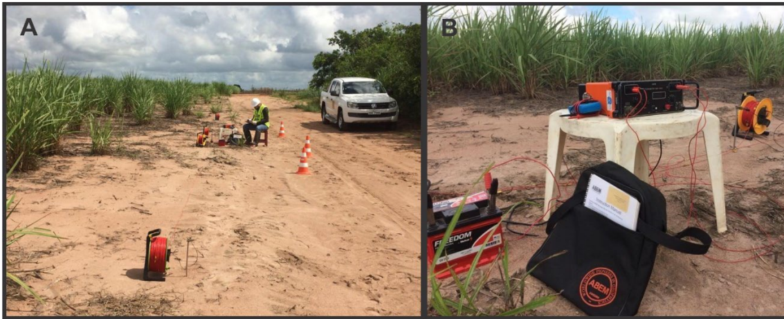
Figure 4 - Aspects of field data acquisition, with Schlumberger electrode array (A) and the used Terrameter SAS 300C resistivity meter (B).
