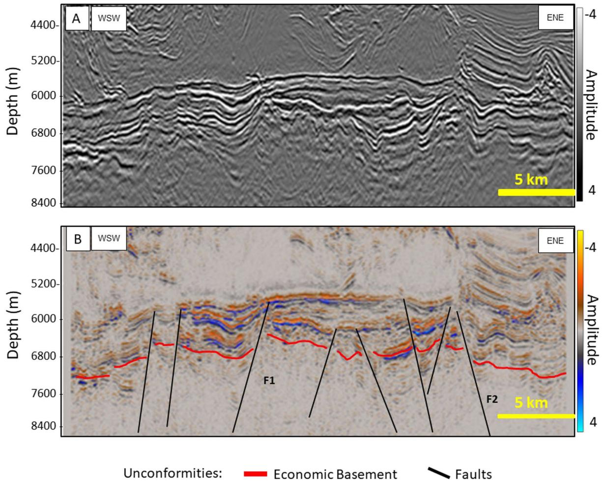
**Figure 4** - Section AA'. Original Seismic (A) and TecVA attribute (B) with Economic basement (red) and main faults (black) highlighted.
