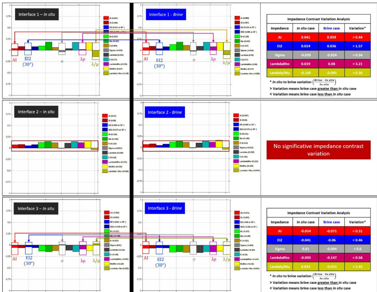
Figure 9 - Elastic contrast analysis showing impedance and elastic modulus variation for fluid scenarios at each interface. The tables at the right of each scenarios display the values for considered impedances and the variation regarding in situ to brine cases.
