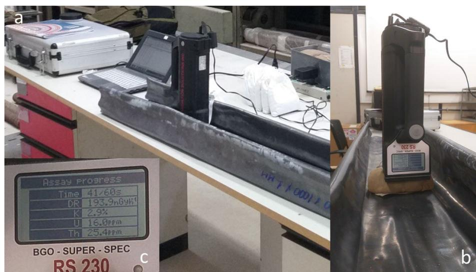
**Figure 2** - a) and b) Acquisition of full and spectral gamma-ray data, from drill cuttings, in a tnt bag, with the portable RS-230 gamma spectrometer, on the lead mesh, at the UFF laboratory. c) Detail of the equipment display (Pereira, 2020).
