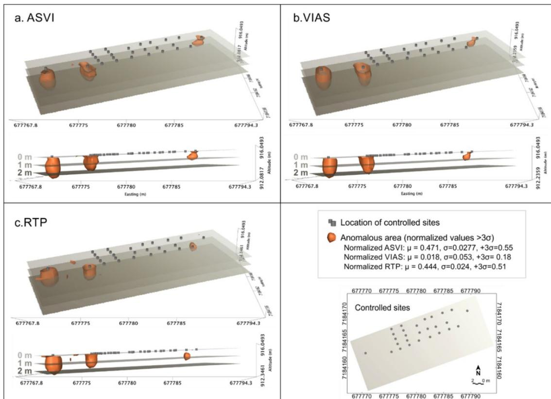
Figure 5: 3D models for the location of Fe-based targets (normalized contrasting susceptibility). Results from the inversion of the ASVI (a), VIAS (b) and RTP (c) data.
