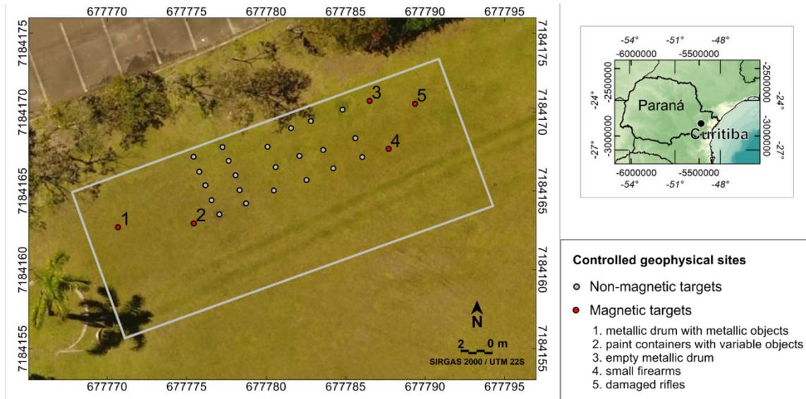
Figure 1: Geophysical test sites in the Polytechnic Center (UFPR), Curitiba, Paraná. The numbers indicate the magnetic test sites. Background image from the Campus Map (Delazari and Ercolin Filho, 2018; <http://www.campusmap.ufpr.br>).
