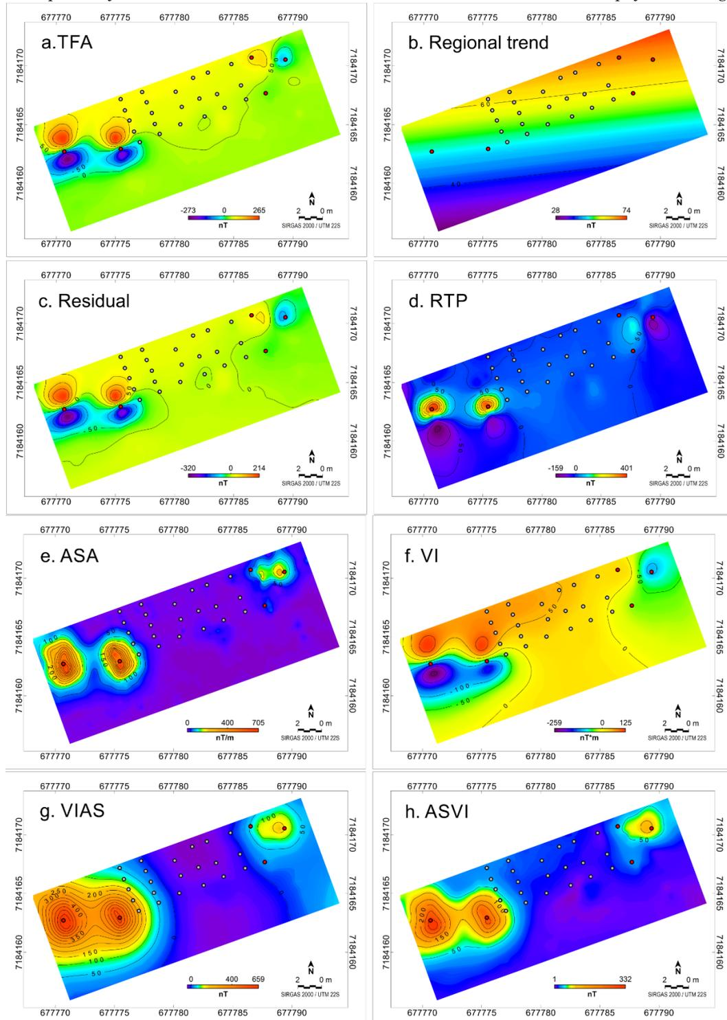
Figure 4: Magnetic data maps. (a) TFA - total field anomaly. Filters applied in the residual TFA grid; (b) Regional trend; (c) Residual; (d) RTP; (e) ASA - analytic signal amplitude; (f) VI - vertical integral; (g) VIAS - vertical integral of the analytic signal amplitude; (h) ASVI - analytic signal amplitude of the vertically integrated field.
