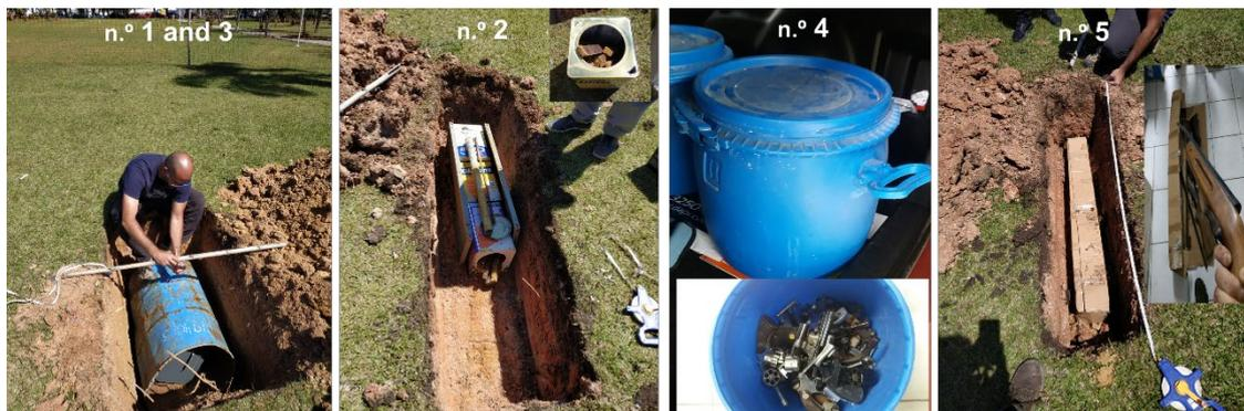
Figure 2: Magnetic materials buried in the controlled sites: 1 and 3 metallic drums with metallic objects and empty, respectively; 2- paint container with varied metallic objects; 4- a plastic drum with small-sized damaged firearms (<20 cm); 5- a pack with damaged rifles.
