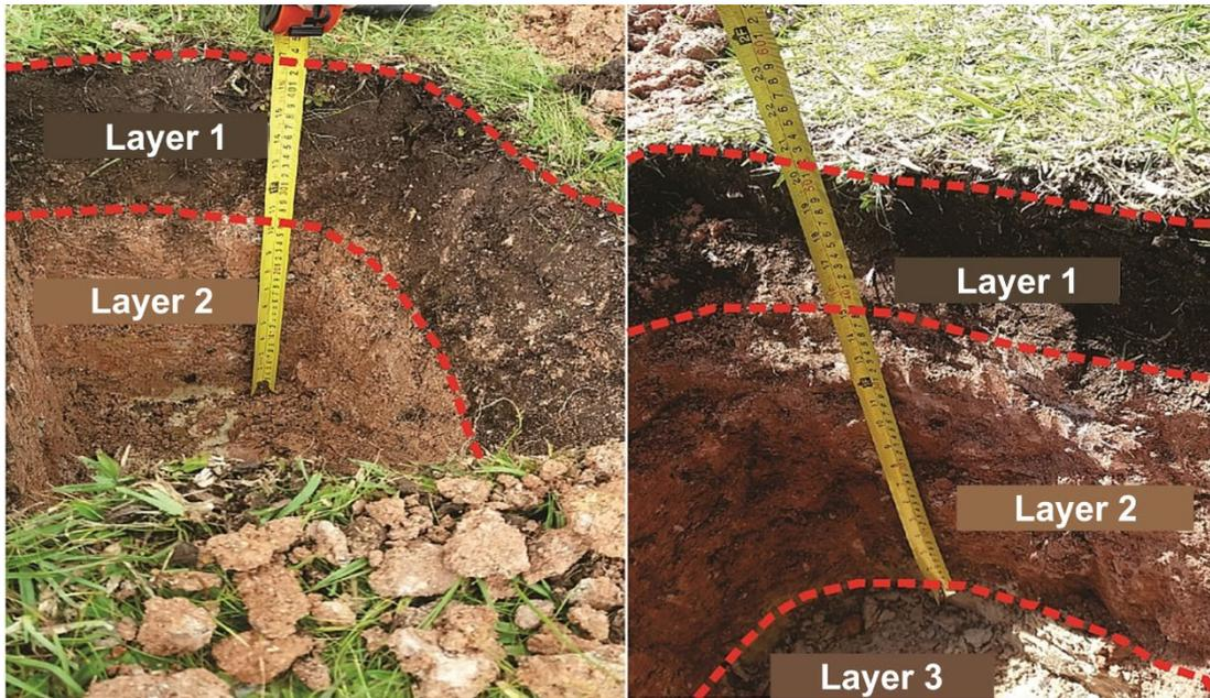
Figure 3: Controlled site soil profile (Canata, 2020). Layer 1: organic soil (0 – 0.2m); Layer 2: clay soil (0.2 – 0.7m); Layer 3: silty soil (0.7 – 1.0m).
