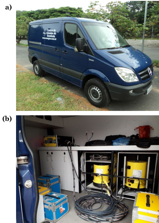
Figure 5: (a) Van used to transport the A10-032; (b) set up of the equipment inside the vehicle.
