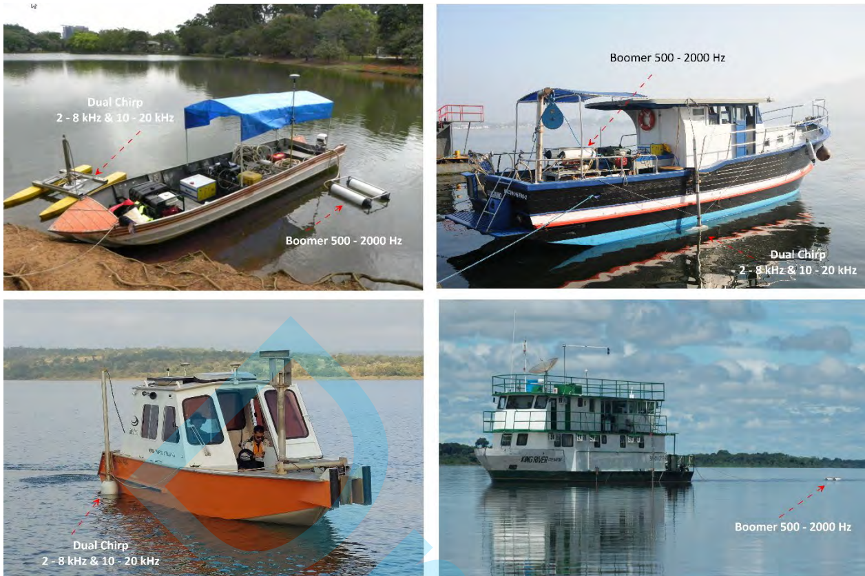
Figure 3: Examples of small boats used for continuous seismic profiling in shallow waters. Top left: small IPT's boat operating at a small lake in São Paulo, with a boomer and a dual chirp. Top right: boat of opportunity with a boomer and a dual chirp at Santos harbor. Bottom left: RuralTech's boat with a dual chirp at Três Marias water reservoir (Minas Gerais State). Bottom right: an Ahitar's boat (local government agency for hydro ways) with a boomer and single chirp (not visible in this photo) in the Araguaia River.
