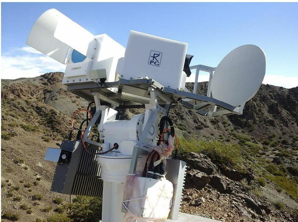
Figure 4: The POEMAS telescope at CASLEO Observatory in Argentina. The 44cm diameter antenna for the 45 GHz receiver is seen on the right of the image, whereas the 90 GHz telescope utilizes a 16.5 cm diameter lens, seen on the left (from [Hidalgo Ramírez et al., 2019](#)).
