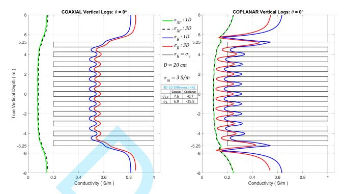
Figure 4. Comparison between 1D and 3D logs, respectively without and with the influence of a borehole in a vertical well in an isotropic shale-sand laminated formation.
