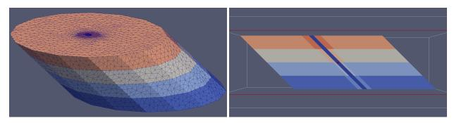
Figure 2. Illustration of the 3D tetrahedral mesh generated with Tetgen. Left: central horizontal slice showing the cylindrical shape of the mesh's outer boundary. Right: vertical slice showing the central well and invasion zones.
