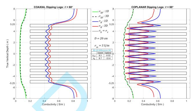
Figure 5. Comparison between 1D and 3D logs, respectively without and with the influence of a borehole in a dipping well at 60° in an isotropic shale-sand laminated formation.
