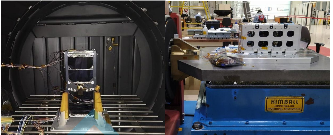
Figure 4: The NANO-SATC-BR2 mounted with several internal and external thermocouples inside the Thermal Vacuum Chamber (left), and the CubeSat placed inside a Test-POD on a shaker at the Integration and Testing Laboratory (right) (Asencio, 2021).
