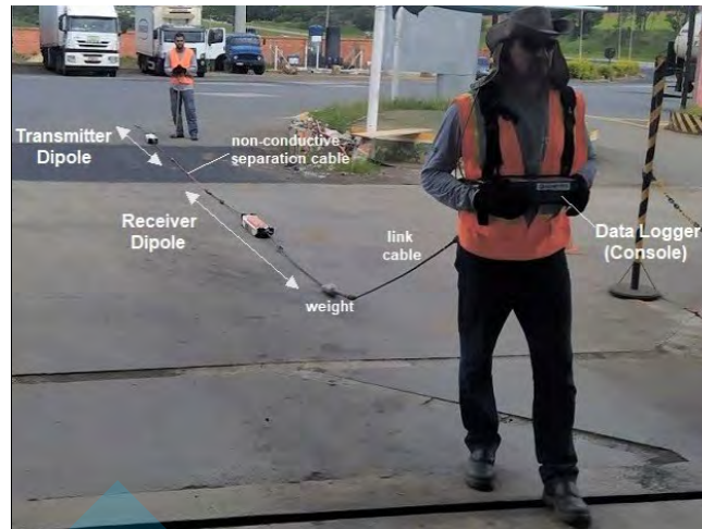
Figure 7 - Ohmmapper TR1 capacitive resistivity meter used. Source: the authors.
