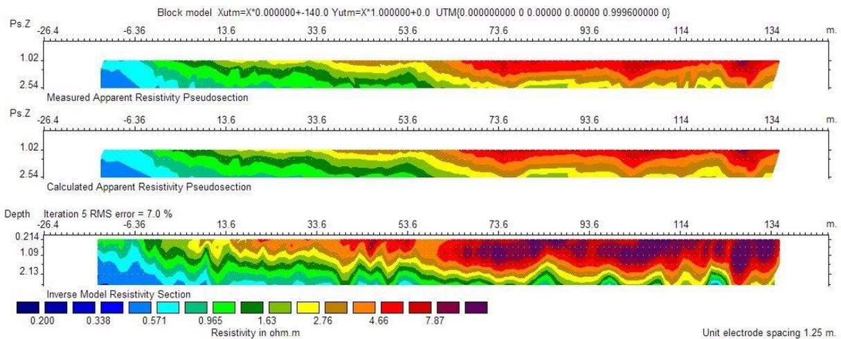
Figure 9: Inversion result of Line 1 with cables of 10 meters: resistivity model (bottom), apparent resistivity values calculated from the resistivity model (middle) and measured apparent resistivity values (top).
