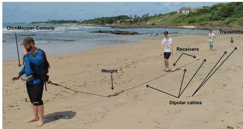
Figure 5: OhmMapper System working with the 5 meters dipolar cable.
