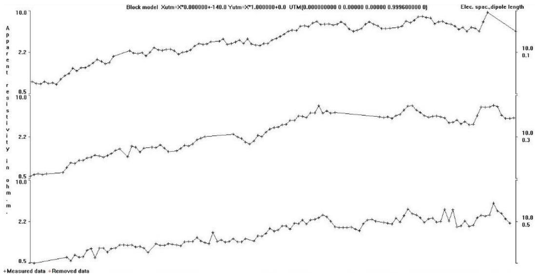
Figure 8: Raw data of apparent resistivity of Line 1 with cables of 10 meters.
