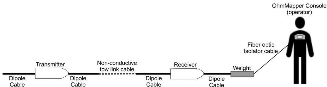
Figure 3: Schematic setup of OhmMapper System. The system can be configured to record data in a discrete or continuous setting, as the operator moves along the survey.
