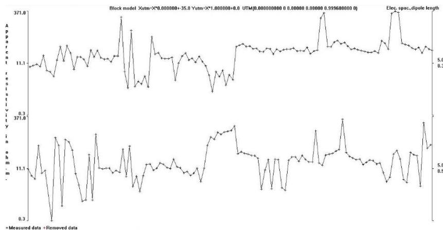
Figure 6: Raw data of apparent resistivity of Line 1 with 5-meter cables. RES2Dinv (Geotomo Software, 2007) raw data visualization tool, in which it is possible to visualize noisy data and delete it.
