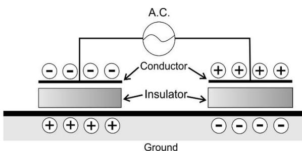
Figure 2: Conceptual model of capacitive coupling of the CR method (modified by Yamashita et al., 2004). Its fundamental difference with respect to the DC resistivity system is that there is no galvanic coupling of electrodes with the soil. The coupling, in this case, is granted by electrical capacitance.
