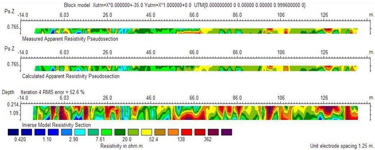
Figure 7: Inversion result of Line 1 with 5-meter cables: resistivity model (bottom), apparent resistivity values calculated from the resistivity model (middle) and measured apparent resistivity values (top).
