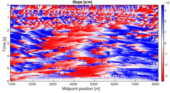
Figure 15: Estimated slopes related to diffraction responses obtained by the diffraction traveltime (equation 1).
