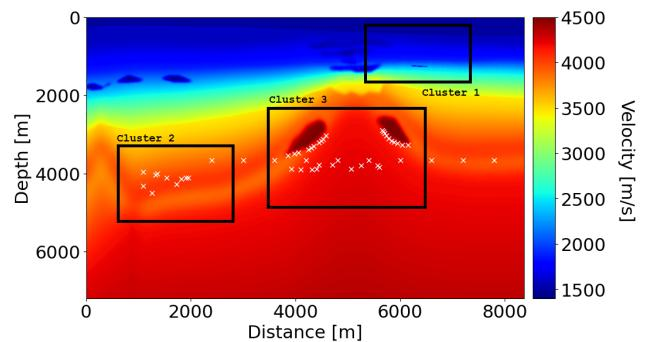
Figure 10: P-wave velocity (BP model). The white times (x) indicate the diffraction points added to the model to validate the proposed method. The regions in the boxes contain the clusters of the target regions where diffractions were picked for the experiments.
