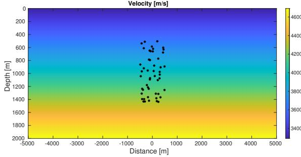
Figure 2: A cluster of diffraction points represented by the black asterisks in a heterogeneous medium with velocities  $V_p = 3292 + 0.7z$  [m/s] and  $V_s = 1768$  [m/s]. A similar cluster configuration is considered for other velocity backgrounds.
