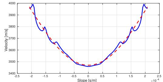
Figure 6: Average D-velocity response (solid blue line) of a diffraction cluster (extracted in the anisotropic target region) embedded in the VTI medium where the first half is isotropic and the second half is the Green River Shale model. The velocity model is described in Figure 2. The red dashed line represents the best fitting using equation 12.
