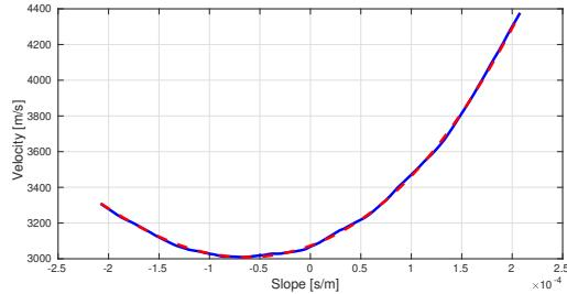
Figure 8: Average D-velocity response (solid blue line) of a diffraction cluster embedded in the VTI medium with  $\epsilon = 0.195$ ,  $\delta = -0.220$  and velocity described in Figure 7. The red dashed line represents the best fitting using equation 12.
