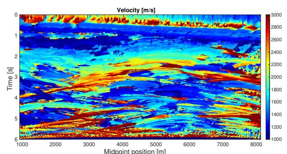
Figure 14: Estimated velocities related to diffraction responses obtained by the diffraction traveltime (equation 1).
