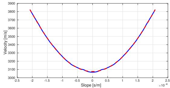
Figure 3: Average D-velocity response (solid blue line) of a diffraction cluster embedded in the VTI medium with  $\epsilon = 0.195$ ,  $\delta = -0.220$  and velocity described in Figure 2. The red dashed line represents the best-fitting parameters using equation 12. The estimated anisotropic parameters are  $\epsilon_E = 0.2163$  and  $\delta_E = -0.1214$ .
