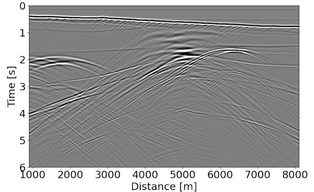
Figure 13: ZO section obtained through finite differences modeling considering the velocity model and Thomsen's parameters shown in Figures 10, 11 and 12.
