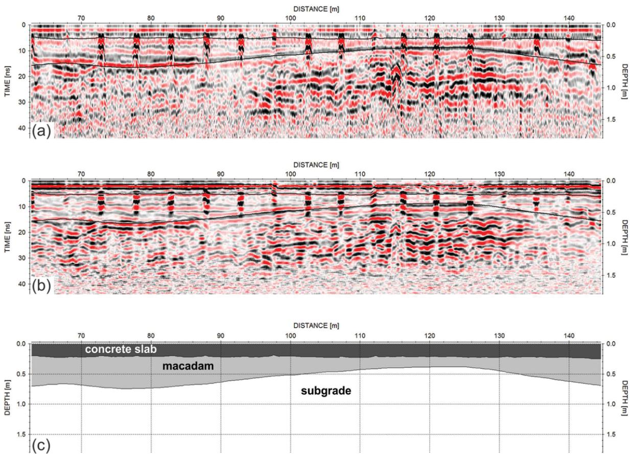
**Figure 8** – GPR sections of L2E, obtained with antennas of (a) 250 MHz and (b) 700 MHz, with geotechnical interfaces model superimposed. (c) Geological and geotechnical model obtained after the interpretation of the GPR sections.
