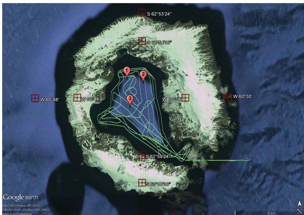
Figure 3 – The multibeam and seismic lines acquired at Port Foster and location of the 3 geological samples acquired (red markers).
