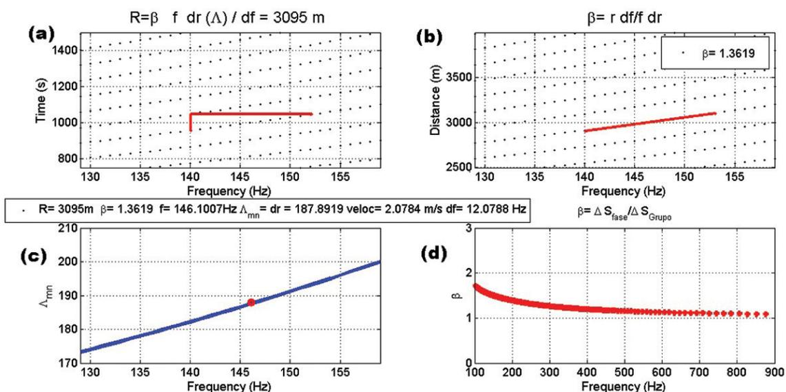
**Figure 3** – Passive distance technique. (a) Spectrogram. (b) Frequency-distance plane. (c) Interference Wavelength. (d)  $\beta$ .
