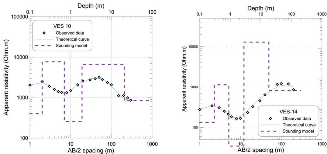
Figure 7 – Examples of representative electrical soundings obtained in this case study.
