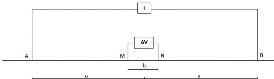
Figure 3 – Sketch of the Schlumberger electrode array.
