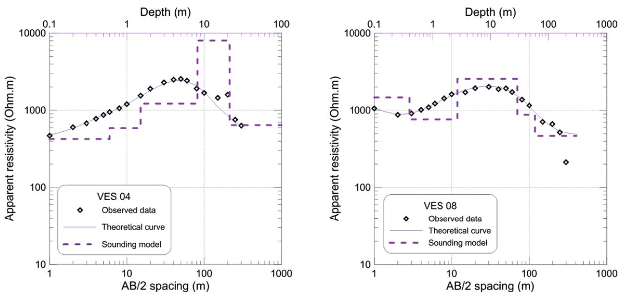
Figure 6 – Examples of representative electrical soundings obtained in this case study.
