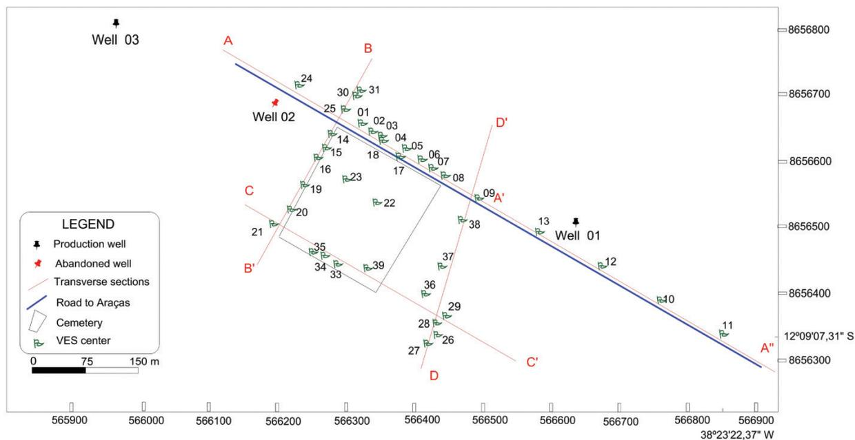
Figure 4 – VES center distribution and the four transverse lines used to depict geoelectrical cross-sections.
