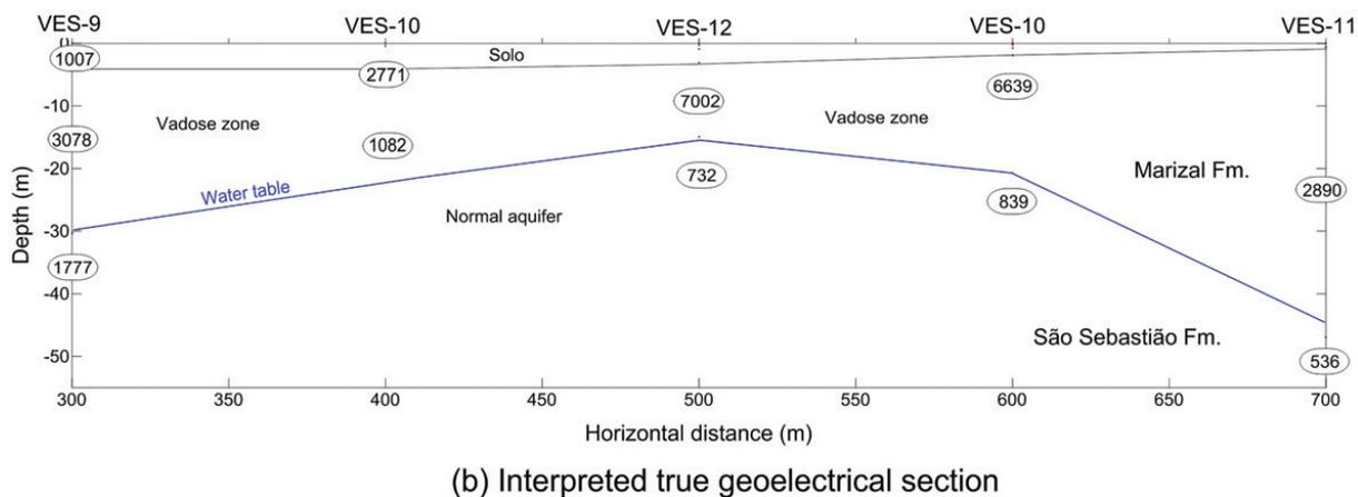
Figure 9 – Apparent resistivity pseudo-section and interpreted geoelectrical section along transverse A' – A".
