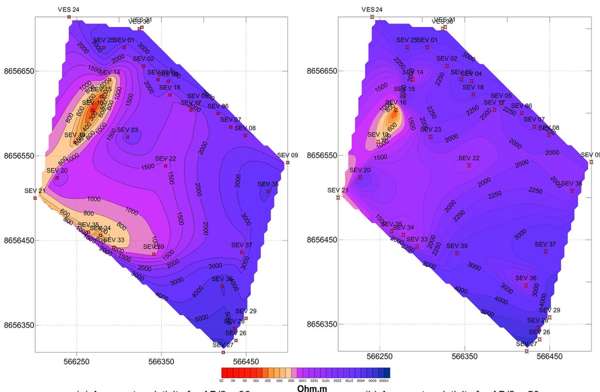
(a) Apparent resistivity for AB/2 = 30 m
