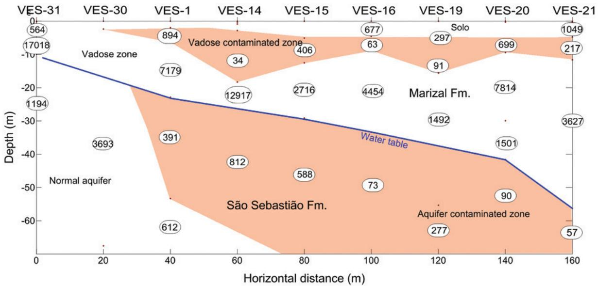
Figure 10 – Apparent resistivity pseudo-section and interpreted geoelectrical section along transverse B – B'.
