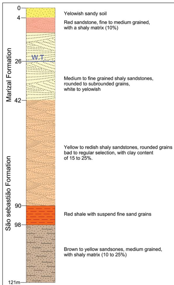
**Figure 2** – Lithological log from well P-3 supplied by SAAE of Alagoinhas.
