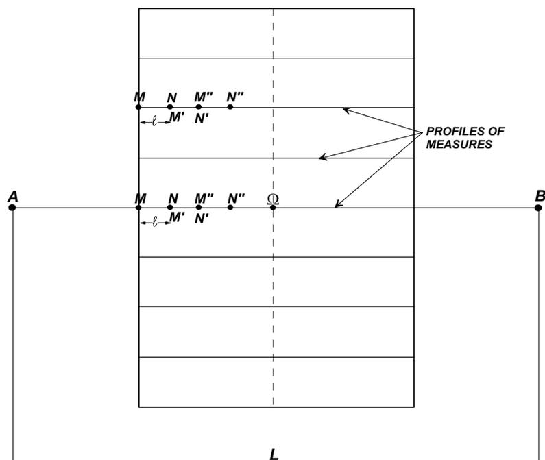
Figure 5 – Gradient or Rectangle Array (Gallas, 2000).
