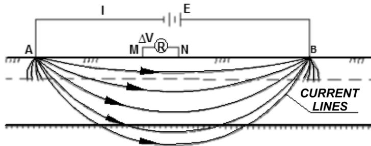
Figure 2 – Principle of Electrical Resistivity Method.
