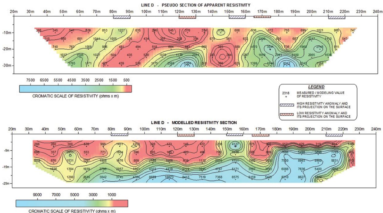
Figure 9 – Modeled resistivity pseudosection and section, D Line.
