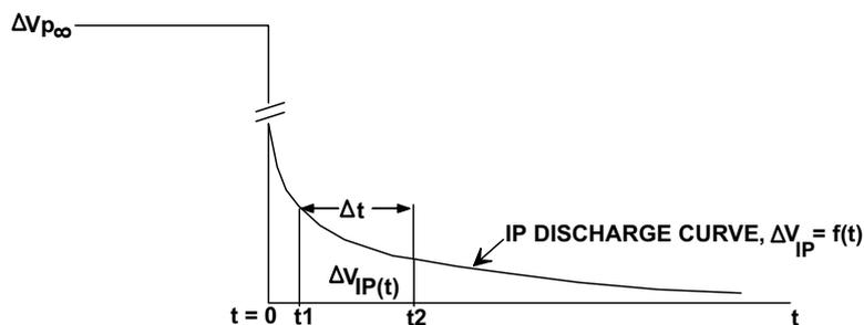
Figure 1 – IP Discharge Curve (adapted from Bertin & Loeb, 1976).
