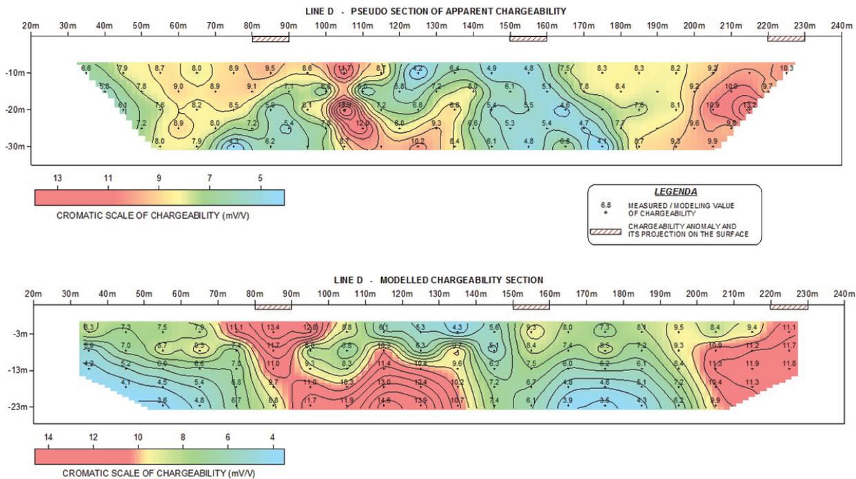
Figure 10 – Modeled chargeability pseudosection and section, D Line.
