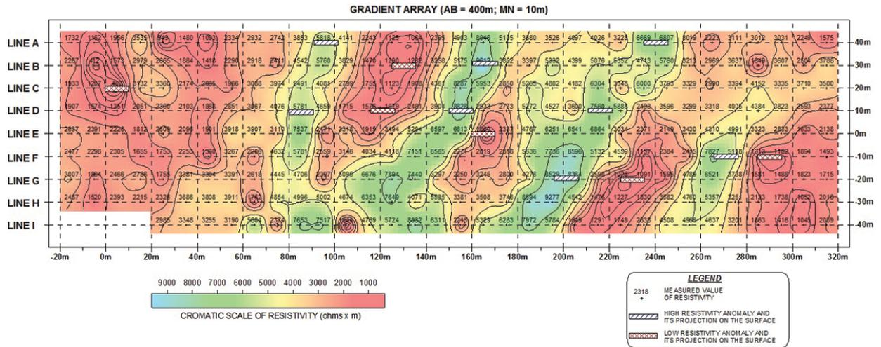
Figure 7 – Map of resistivity, gradient 1 + gradient 2.
