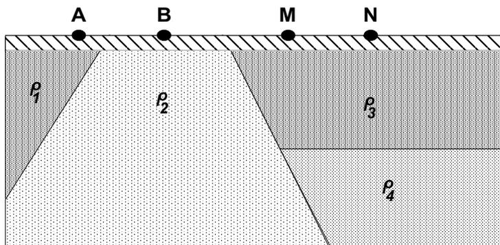
Figure 3 – Heterogeneous Substrate (Gallas, 2000, modified from Orellana, 1972).
