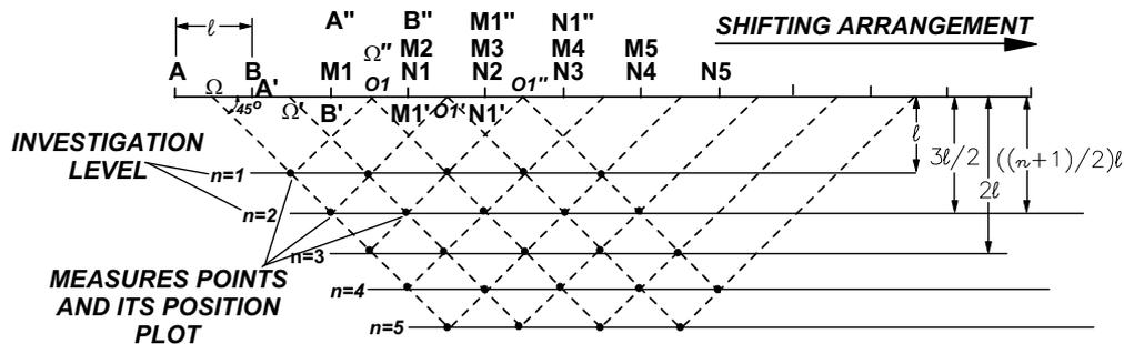
Figure 4 – IP-Resistivity Profiling/Disposition in dipole-dipole array field (Gallas, 2000).
