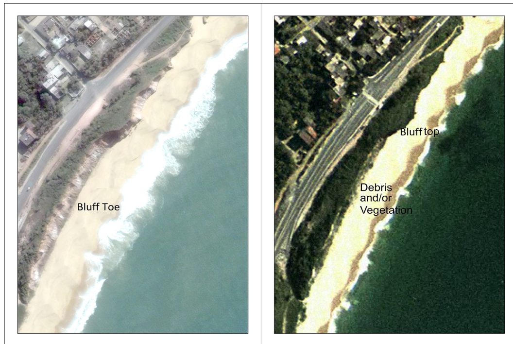
Figure 4 – Adaptation to extract bluff toe as a shoreline proxy from images. Satellite photos from Google Earth.
